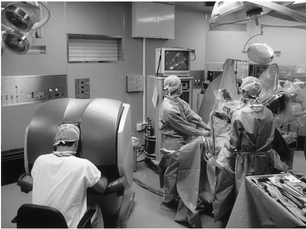
Fig. 3 Operation using a master-slave manipulator.
